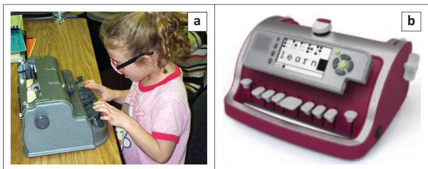
FIGURE 7.15: (a) Traditional brailier and (b) new brailier with screen.
